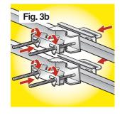
5) Attach the Combiner Bars (5) to each terminal on the back of each Loop Element (4) as shown. There are two attachments on each Loop Element. Secure loosely with the Wing Nuts (11), do not over tighten. Fig. 4
