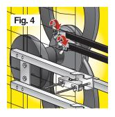
Mast Clamps (12) onto the Mast. Tighten the Wing Nuts (13) to secure the antenna to the Mast. Place Mount Base End Cap (8) onto the J-Mount Mast (6).
