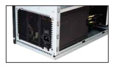
Unique Power Supply Option: Comes with a power supply mounting adapter to mount either a regular PS/2 size power supply or the unique Antec CP-850 or CP-1000 super quiet, high performance power supply
