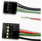
3. Working carefully so as not to damage the wires, connectors or pins, slowly reinsert the pin into the correct slot of the connector then snap closed the black tab that was lifted in step 1. Repeat these steps for each wire you need to change.
