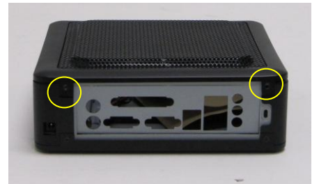
Remove these case screws
