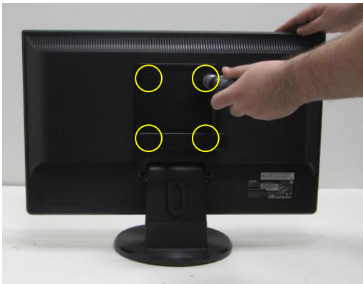
Attach the mount with the four included screws
