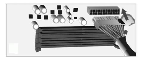
Connect the 8-pin or 4+4-pin connector for the CPU. If your motherboard has an 8-pin socket with a cover on some of the openings, we recommend that you remove the cover and use the 8-pin connector.
