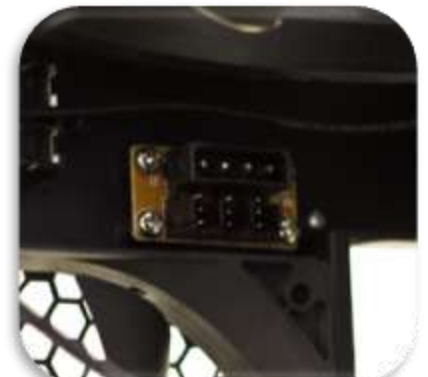
Reinstall the power hub in the correct orientation.
