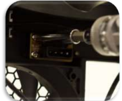
Loosen the power hub by removing the four screws.
