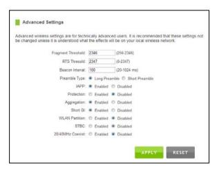
Preamble Type: Defines the length of the Cyclic Redundancy Check for communication between the Range Extender and roaming Wi-Fi users.
