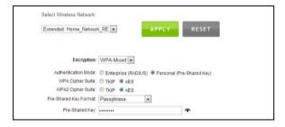
Using the drop down menu, you can select which network you wish to configure and may adjust the security settings below.
