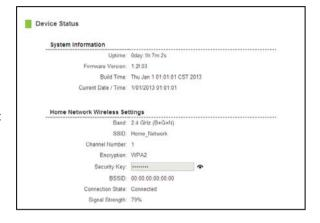
Home Wi-Fi Network Settings: This section displays the current status of the connection between the Range Extender and your Home Network. When viewing this section, it is important to check that your Home Network SSID is correct and the channel number matches your Home Network's channel number settings.
