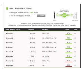
The Scan results page will display information regarding the name of the network (SSID), the channel which the Wi-Fi network is operating on and the security type of network. The results page will also display what the signal strength is coming from each specific network detected.
