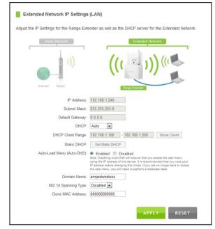
DHCP Client Range: The range of IP addresses the Range Extender's DHCP server will assign to users and devices connecting to the Range Extender.
