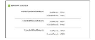
Extended Wired Network: The Wired Connection statistics shows all data activity for all users physically connected to the wired ports on the Range Extender.
