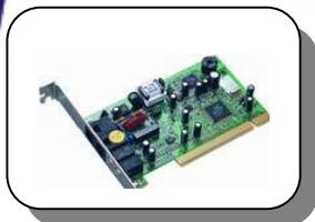
AMI-IA56 & AMI-IE56, Intel's Host Accelerated Modem (Controller-Less) solution with complete set
