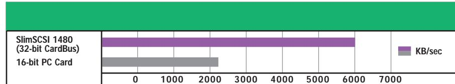
Adaptec 16-bit SlimSCSI 1460 vs. Adaptec 32-bit SlimSCSI 1480 adapter.
