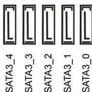
These five SATA3 connectors support SATA data cables for internal storage devices with up to 6.0 Gb/s data transfer rate.
