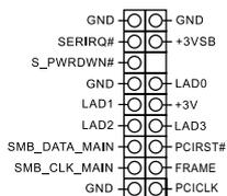
This connector supports Trusted Platform Module (TPM) system, which can securely store keys, digital certificates, passwords, and data. A TPM system also helps enhance network security, protects digital identities, and ensures platform integrity.
