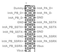
Besides four USB 3.0 ports on the I/O panel, there is one header on this motherboard. Each USB 3.0 header can support two ports.
