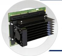
5A Dual Core Processor Board (No. CPU-5A-C21) Processor/Socket: Dual-core 64-bit 3400e Speed: 1.8GHz Memory: 2GB DDR2 L2 Cache: 1MB Power: 20 Watts Interface: HT3-1GHz
