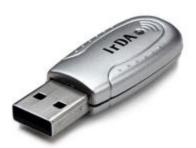
The USB2IR3 USB to IR Adapter turns a USB port into an IrDA compliant infrared port for communication with a wide variety of IrDA compliant devices, such as PDAs, cell phones, test equipment and medical instruments.
