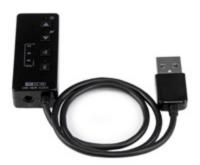
The ICUSBAUDIOMH External USB Card lets you add an S/PDIF digital audio output or a standard 3.5mm analog audio connection to your system through USB. By converting a single USB port into an external sound card with microphone connectivity, you can conveniently bypass or replace an internal sound card without having to open your computer case.
