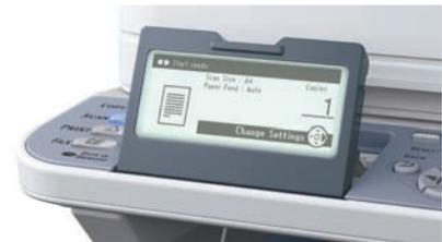
**Backlit LCD display:** tilts up as much as 90°.
