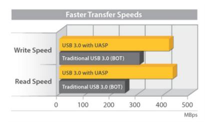
At the same peak in testing UASP also shows an 80% reduction in required processor resources.
