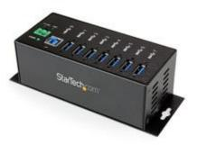
The ST7300USBM Industrial 7-Port USB 3.0 Hub expands your current USB capability by adding 7 external USB 3.0 ports from a single USB 3.0 host connection, powered via a 2-wire terminal block supporting a wide-range 7–40V DC input.
