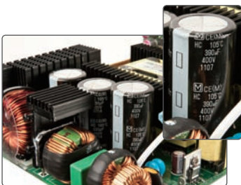
Solid State Capacitors and 105°C Japanese Grade A Capacitors
