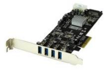
The PEXUSB3S42V 4-Port PCI Express USB 3.0 Card lets you add four USB 3.0 ports with two dedicated 5 Gbps channels to your PCIe x4-enabled PC. This independent port architecture improves USB 3.0 performance by transferring data on two individual channels to your computer, giving you faster file transfers.
