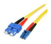
The SMFIBLCSC7 7m LC to SC Single-Mode Duplex Fiber Cable features 9/125 micron fiber for high-speed, high bandwidth data transmissions over Gigabit Ethernet and Fiber Channel networks, with support for duplex single-mode applications.
