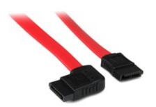
The SATA18RSA1 Right Side-Angled SATA Cable (18-inch) features one straight and one right side-angled (7-pin) data receptacle, which positions the cable so that it runs parallel to the drive ports – ideal for connectivity in narrow spaces, enabling installation of the drive as needed within the system case.
