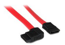
The SATA12RSA1 Right Side-Angled SATA Cable (12-inch) features one straight and one right side-angled (7-pin) data receptacle, which positions the cable so that it runs parallel to the drive ports – ideal for connectivity in narrow spaces, enabling installation of the drive as needed within the system case.
