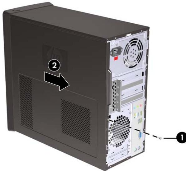
To replace the access panel, reverse the removal steps.
