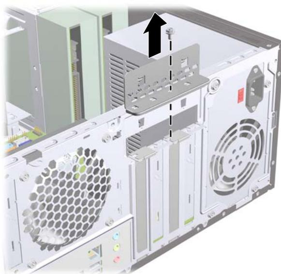
5. Before installing an expansion card, remove the expansion slot cover or the existing expansion card.
