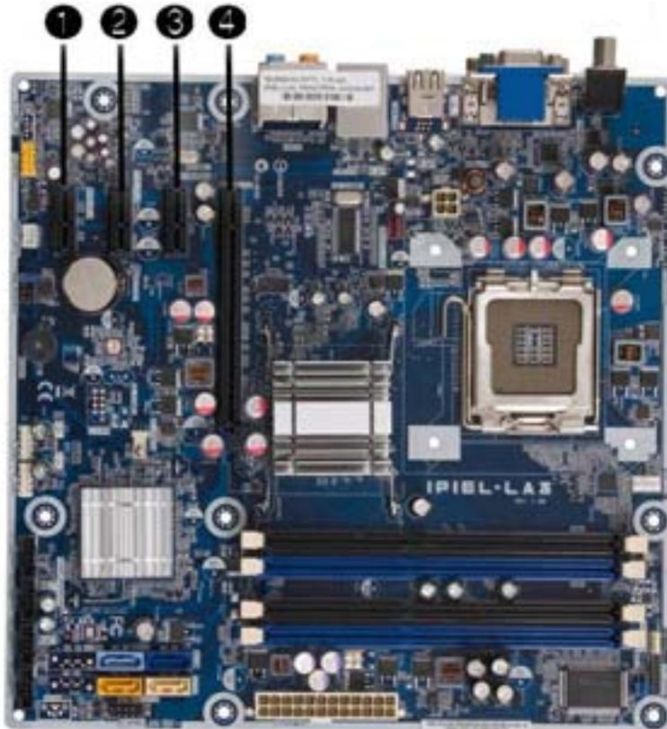
**Figure 6-9** Expansion Slot Locations – HP Pro 3130
