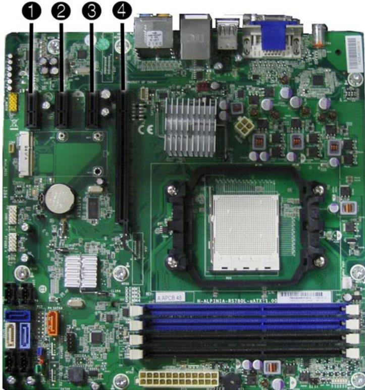
**Figure 5-10** Expansion Slot Locations – HP Pro 3130
