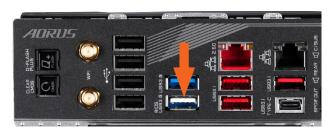
5 Press the Q-Flash Plus button (location may vary by model) and the system will automatically search and match the BIOS file in the USB flash drive on the white USB port. The QFLED and the Q-Flash Plus button on the rear panel will flash during the BIOS matching and flashing process. Wait for 2-3 minutes and the QFLED will stop flashing when the BIOS flashing is complete.
