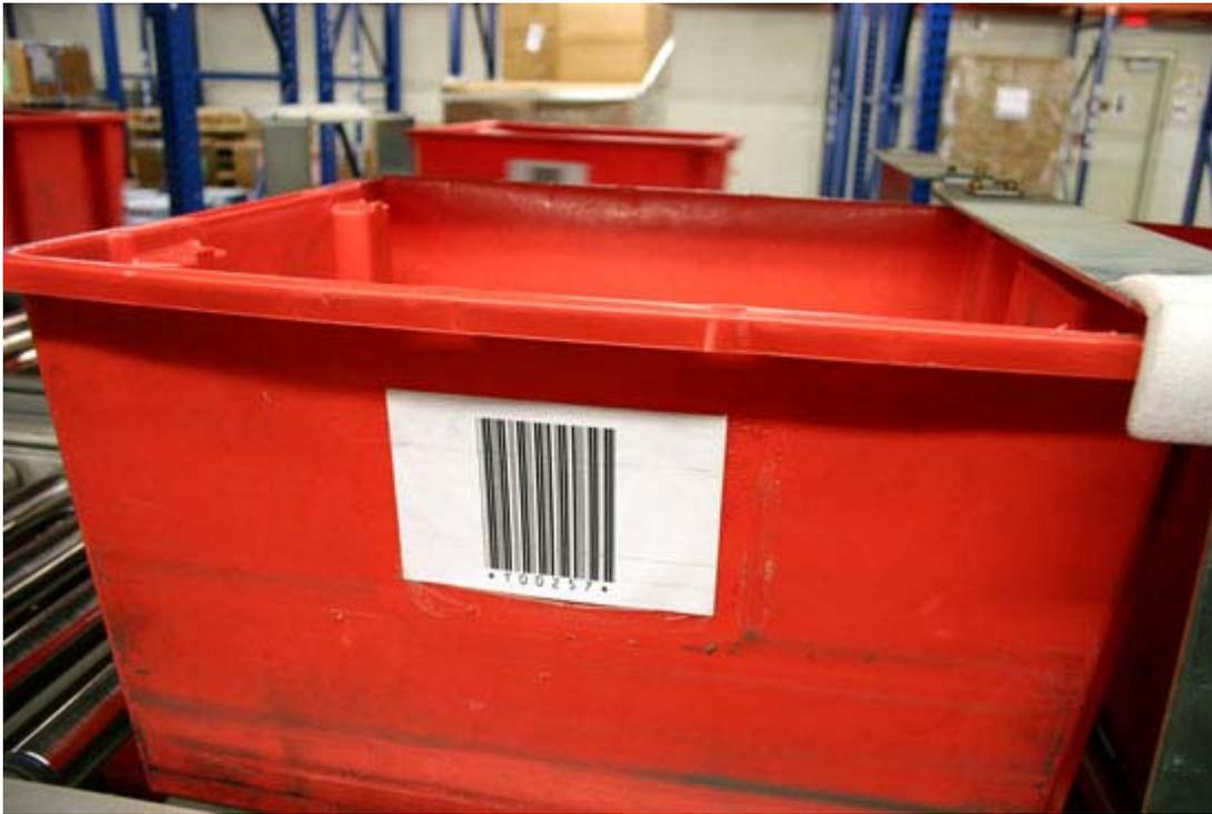
The tub glides along a rolling conveyor, which will carry the tub from the start on the first floor all the way up to the third floor. Along its journey it will pass by Newegg's inventory; the system (pictured below), knowing exactly what your order should contain, will stop the tub whenever it gets to an item that needs to be put into it.
