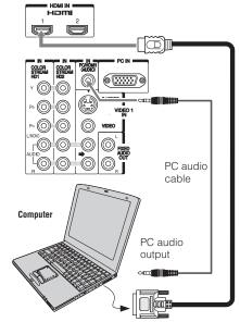
The HDMI input can accept and display VGA, SVGA, XGA, WXGA, SXGA, 480i (60 Hz), 480p (60 Hz), 720p (60 Hz), 1080i (60 Hz), and 1080p (24 Hz/60 Hz) signal formats. For detailed signal specifications, see page 64.
