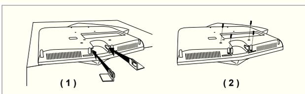
1. When installing the TV on the wall without using the stand, insert decoration covers into the holes as described in the picture (1).
