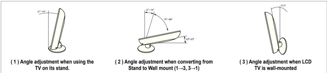
> When you adjust the stand, press the button on the back of the stand.
