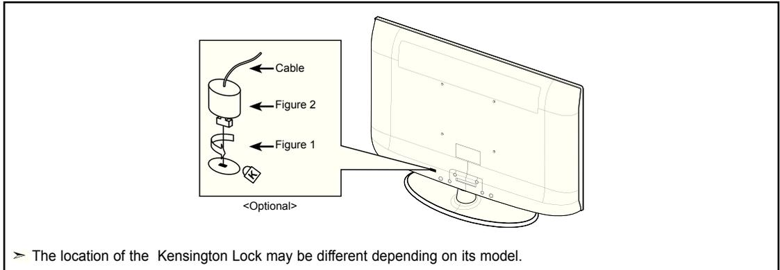
1. Insert the locking device into the Kensington slot on the LCD TV (Figure 1) and turn it in the locking direction (Figure 2).
