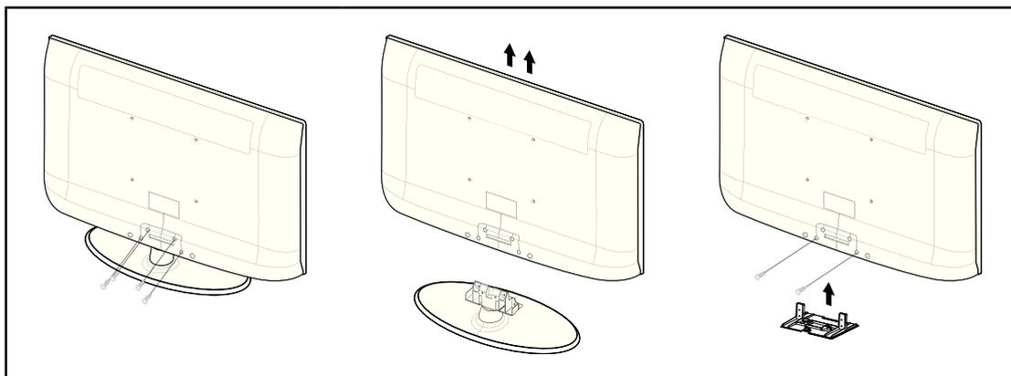
1. Remove four screws from the back of the TV.
