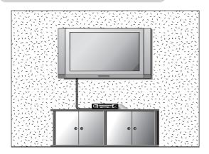
For proper ventilation, allow a clearance of 4" on each side and 2" from the wall. Detailed installation instructions are available from your dealer, see the optional Wall Mounting Bracket Installation.
