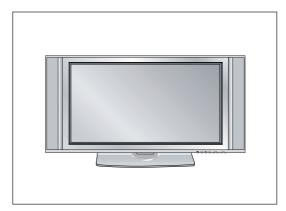
For proper ventilation, allow a clearance of 4" on each side and the top, 2.36" on the bottom, and 2" from the wall. Detailed installation instructions are included in the optional Desktop Stand Installation.
