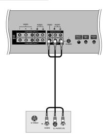
The TV has a special signal output capability which allows you to hook up a second TV or monitor.
