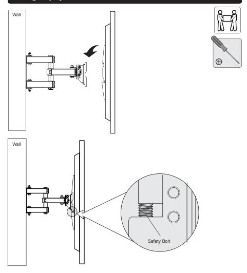
Using an assistant or mechanical lifting equipment, hook the display with attached adapter brackets over the top of the wall mount's arm assembly plate. Tighten the safety bolts on the bottom of the adapter brackets to secure the unit.
