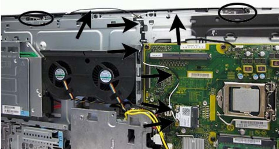
To install the antenna, reverse the removal procedures.
