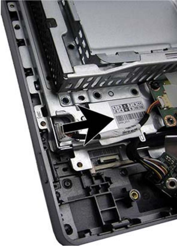
**13.** Separate the display panel from the bezel.
