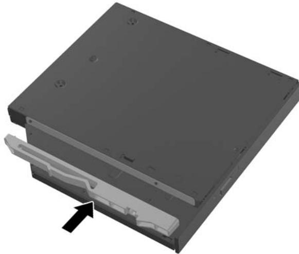
6. Align the new optical disc drive with the opening in the side of the computer. Push the drive in firmly until it snaps into place.
