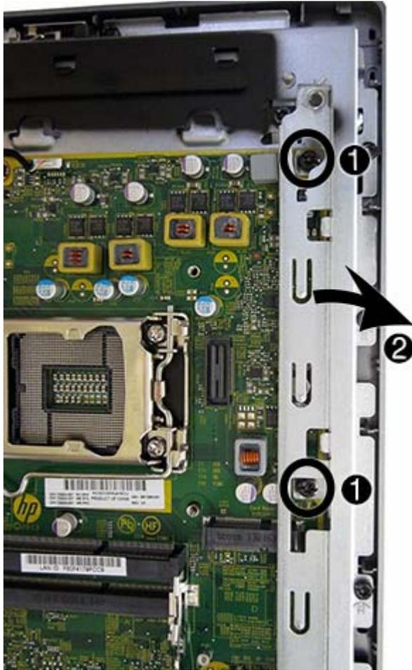
14. Remove the eight remaining Torx screws that secure the system board to the computer.
