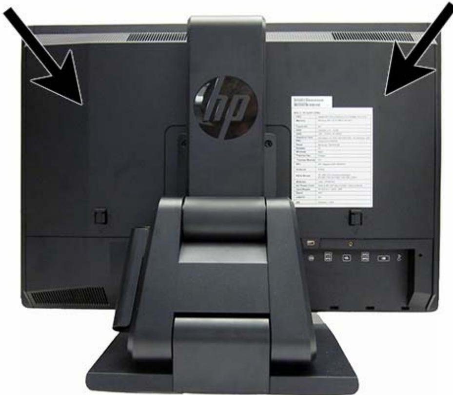
The computer has one main rear access panel that allows access to internal components.
