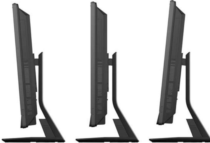
The tilt/swivel stand has a swivel pad on the underside that allows you to swivel the computer up to 360 degrees left or right for the best viewing angle.
