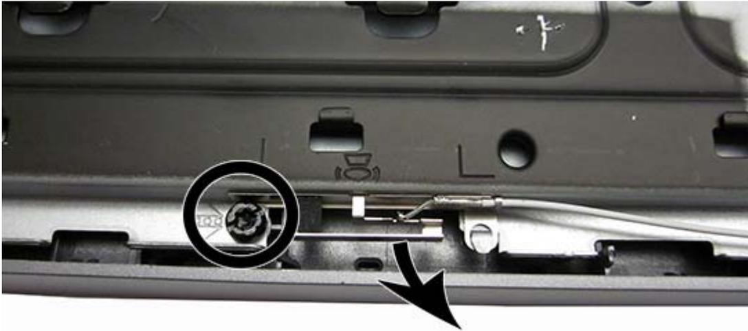
6. Note the routing path for each antenna for replacement.
