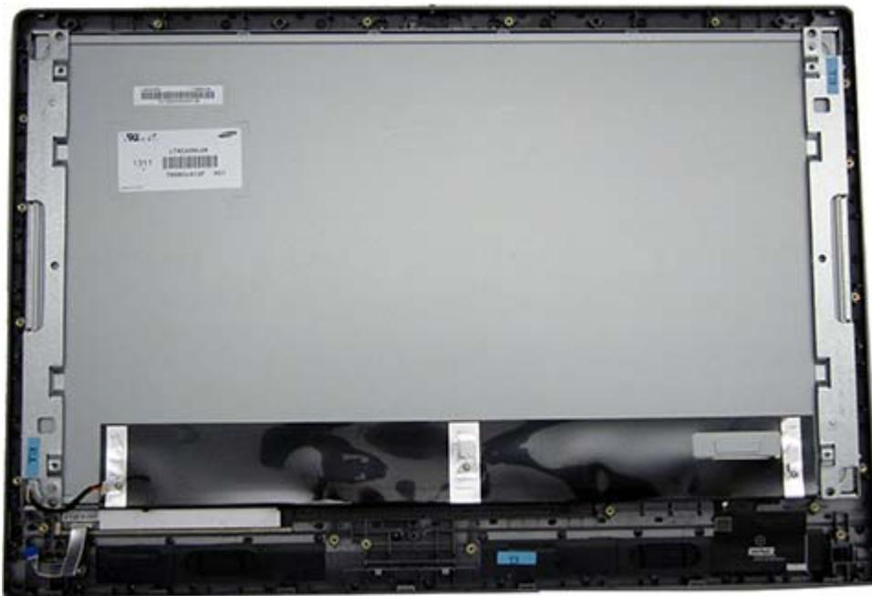
**12.** Disconnect the backlight cable from the display panel.
