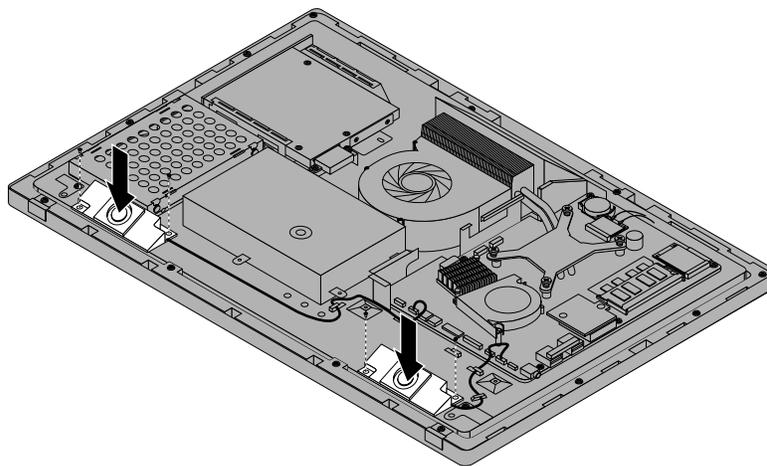
Figure 53. Installing the internal speakers
