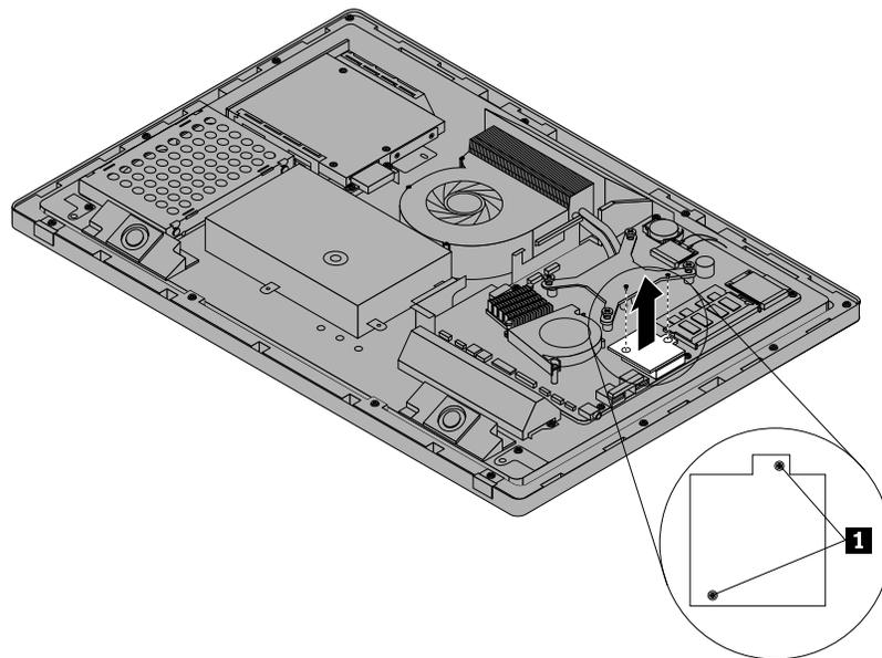
Figure 42. Removing the card reader
