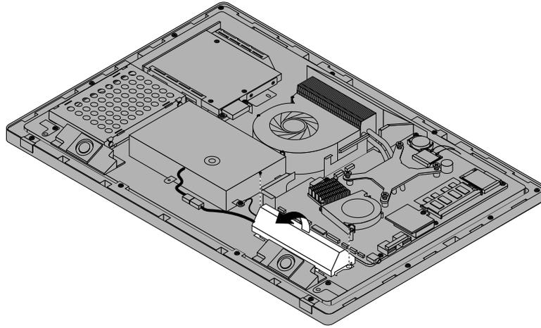
Figure 25. Removing the two screws that secure the rear I/O assembly
