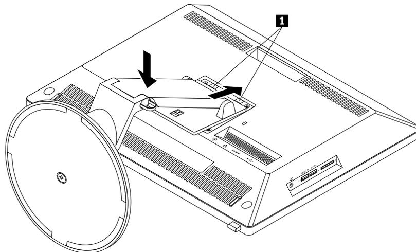
Figure 10. Installing the transformer stand
