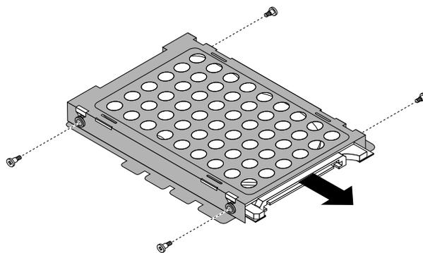
Figure 15. Removing the hard disk drive from the hard disk drive bracket
