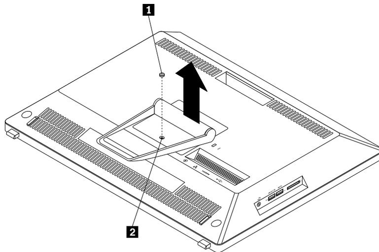
Figure 5. Removing the frame stand
