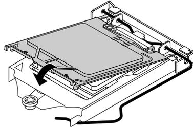
Figure 58. Installing the microprocessor socket cover
