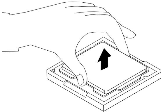
Figure 40. Removing the microprocessor
