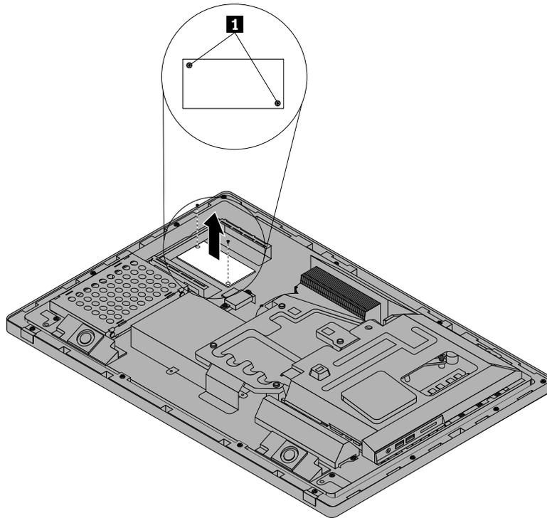
Figure 48. Removing the converter board
