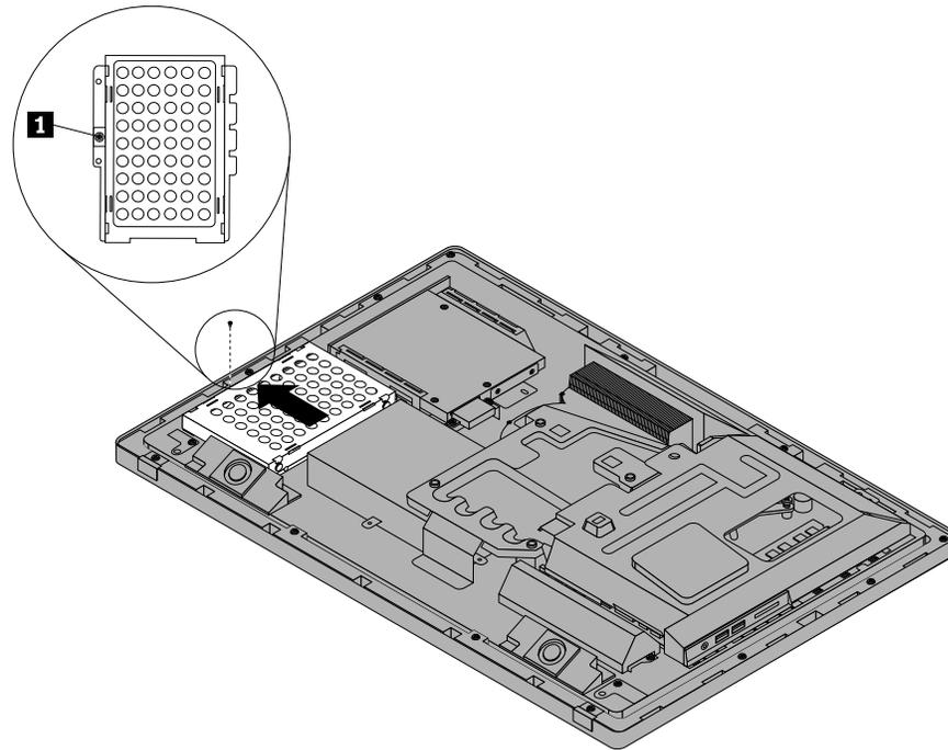
Figure 14. Removing the hard disk drive assembly
