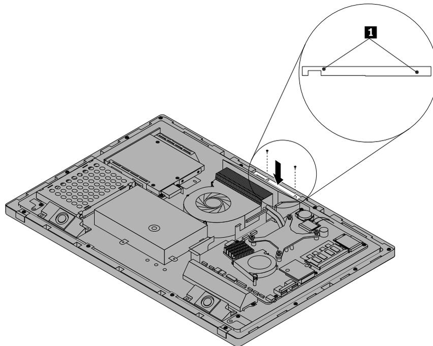
Figure 55. Installing the integrated camera
