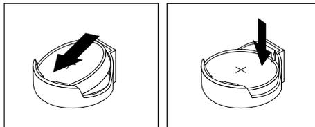
Figure 47. Installing a new battery
