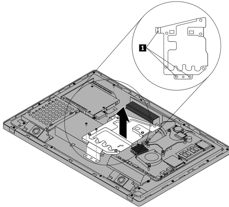
Figure 23. Removing the VESA mount bracket
