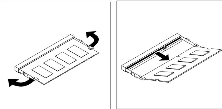
Figure 50. Removing a memory module
