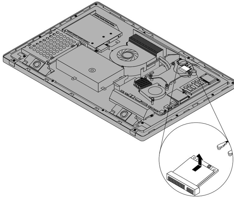
Figure 66. Removing the Wi-Fi card
