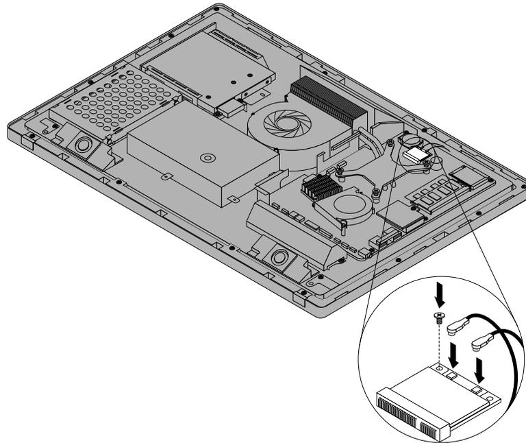
Figure 68. Securing the Wi-Fi card and connecting cables
