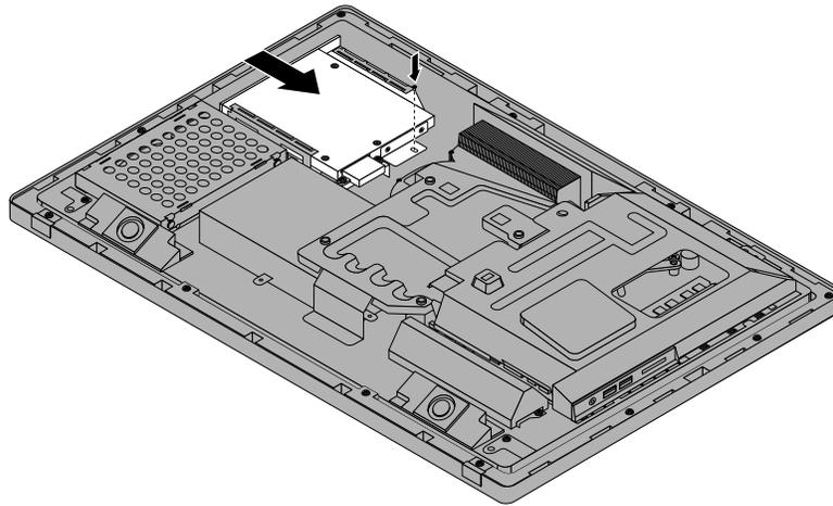
Figure 19. Installing the optical drive
