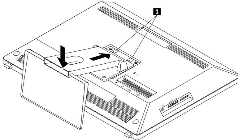
Figure 8. Installing the monitor stand
