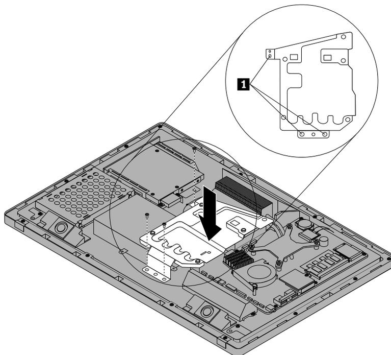
Figure 24. Installing the VESA mount bracket
