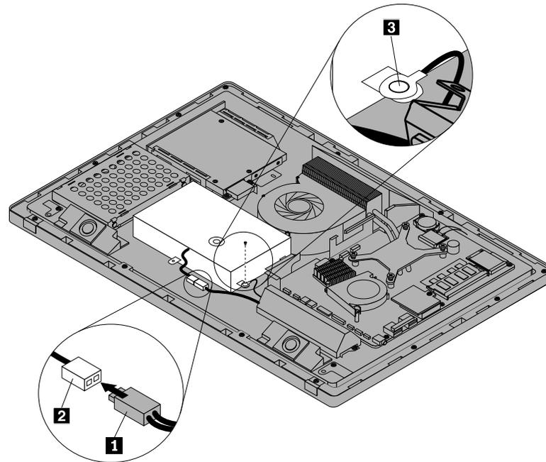
Figure 34. Connecting the power cables and securing the earth wire
