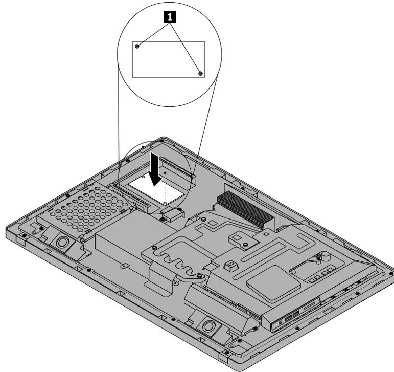
Figure 49. Installing the converter board
