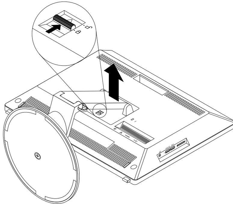
Figure 9. Removing the transformer stand
