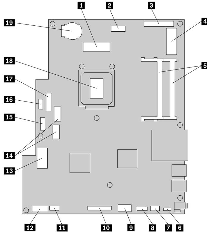
Figure 4. Locations of the parts and connectors on the system board
