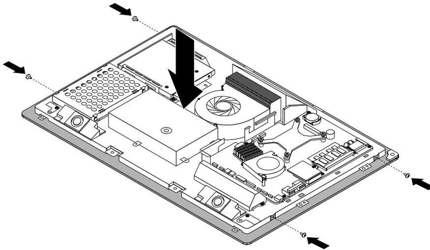
Figure 62. Installing the four screws to secure the LCD panel assembly
