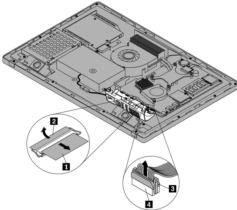
Figure 26. Disconnecting the HDMI and USB cables
