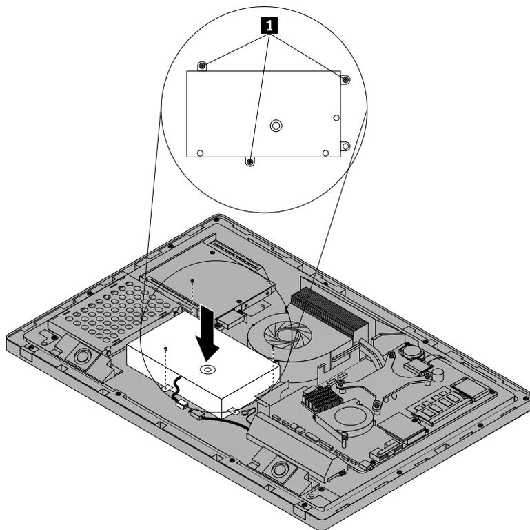
Figure 33. Installing the power supply assembly
