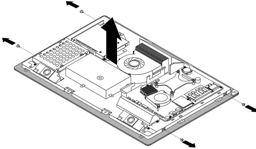
Figure 61. Removing the four screws that secure the LCD panel assembly
