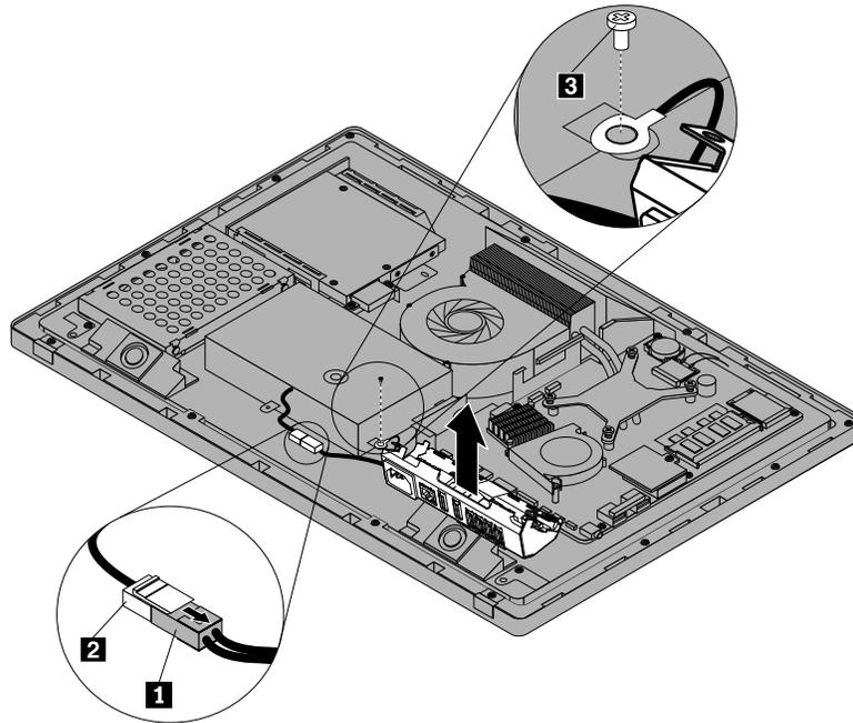
Figure 27. Removing the rear I/O assembly
