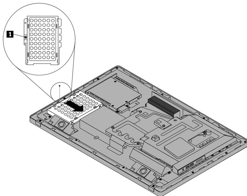
Figure 17. Installing the hard disk drive assembly
