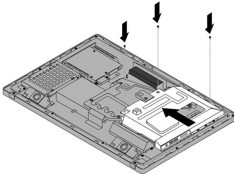
Figure 22. Installing the three screws to secure the system board shield
