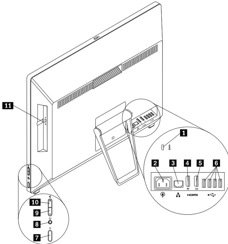
Figure 2. Rear connector locations
