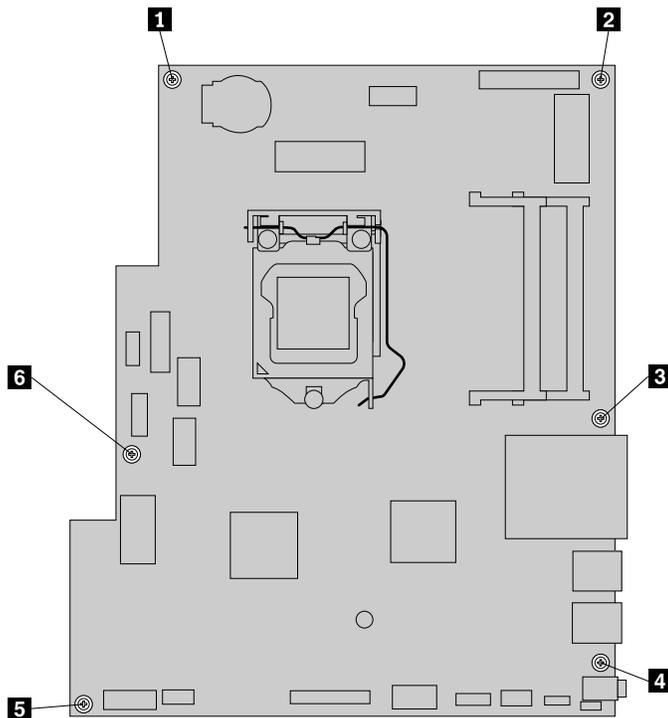
Figure 57. Installing the six screws that secure the system board to the main bracket
