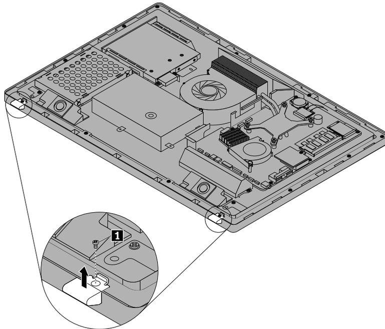
Figure 12. Removing the feet
