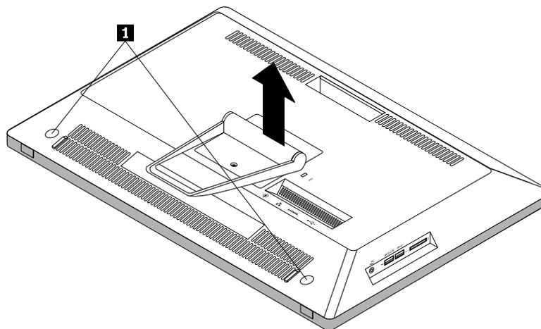
Figure 11. Removing the computer cover
