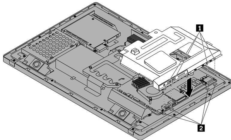
Figure 21. Positioning the system board shield onto the chassis
