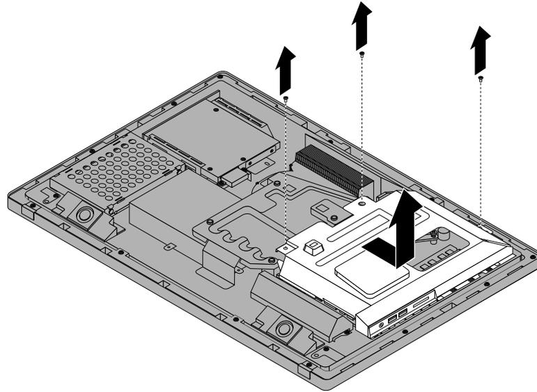
Figure 20. Removing the system board shield
