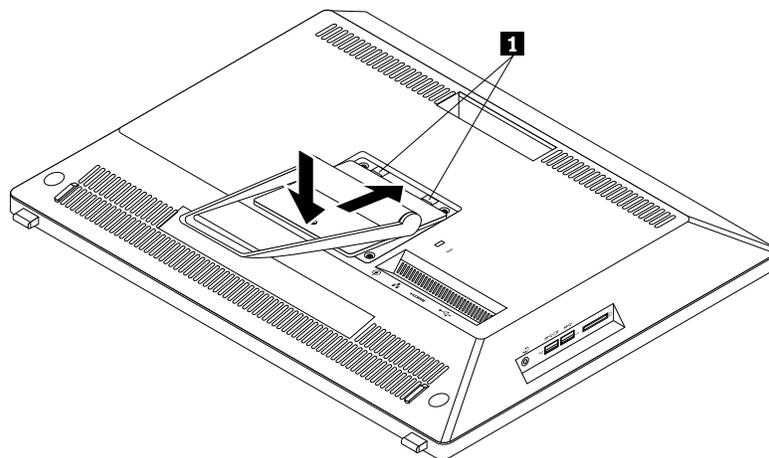
Figure 6. Installing the frame stand
