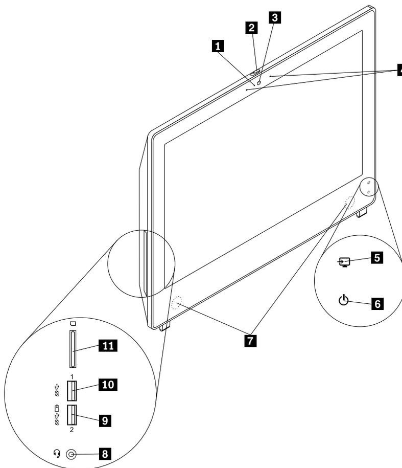
Figure 1. Front connector, control, and indicator locations
