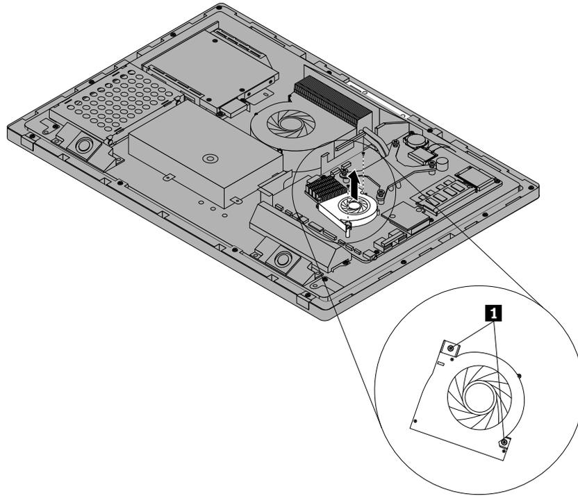
Figure 44. Removing the GPU fan
