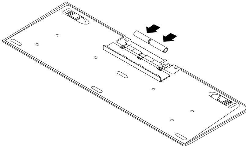
Figure 70. Installing the keyboard batteries
