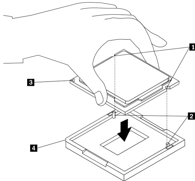
Figure 41. Installing the microprocessor
