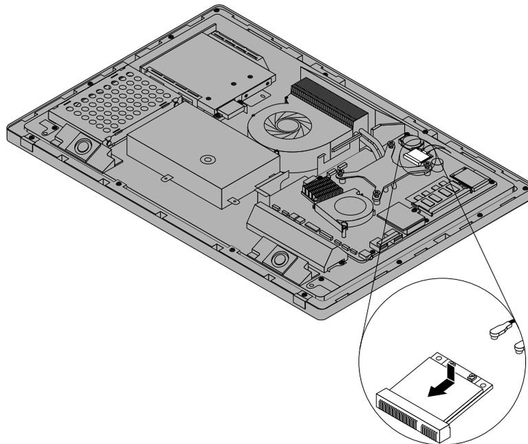
Figure 67. Installing the Wi-Fi card
