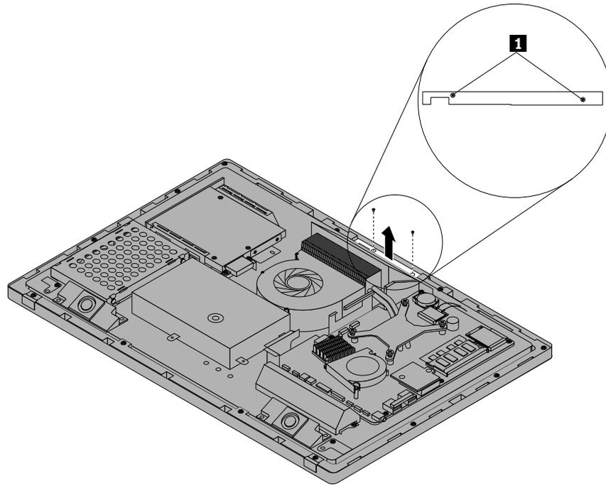
Figure 54. Removing the integrated camera
