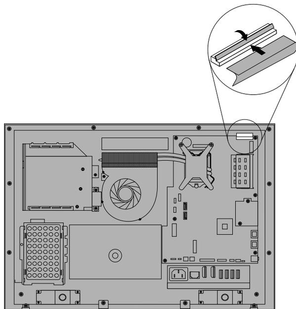
Figure 64. Connecting the LCD panel cable to the system board
