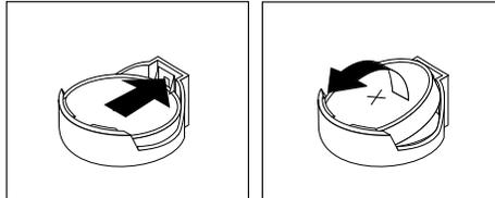
Figure 46. Removing the battery
