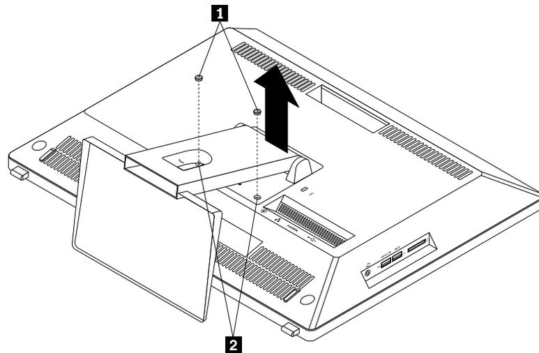
Figure 7. Removing the monitor stand
