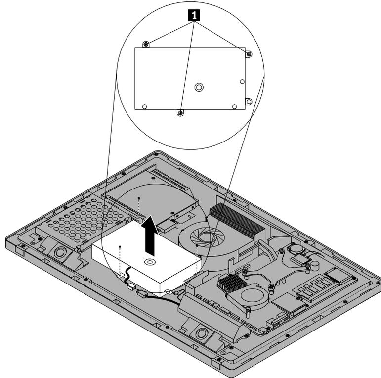
Figure 32. Removing the power supply assembly
