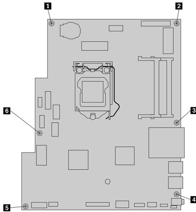
Figure 56. Removing the six screws that secure the system board
