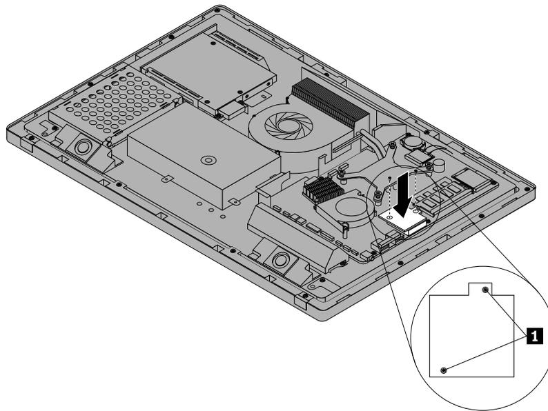
Figure 43. Installing the card reader
