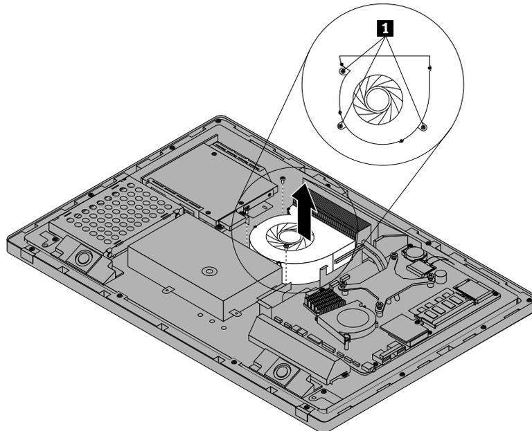
Figure 35. Removing the microprocessor fan
