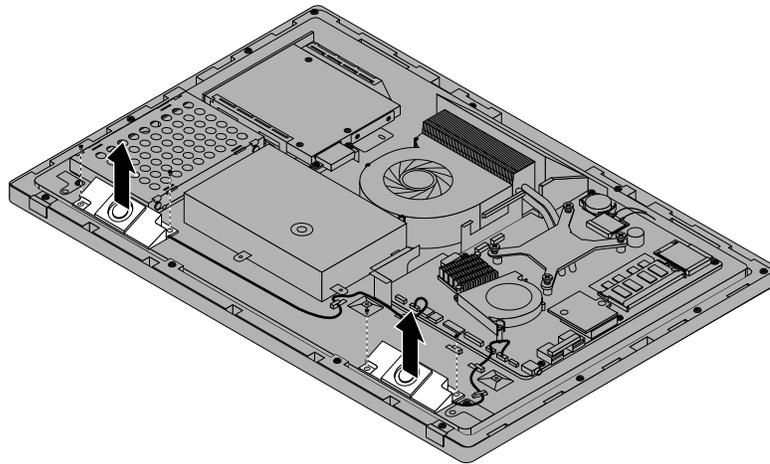
Figure 52. Removing the internal speakers
