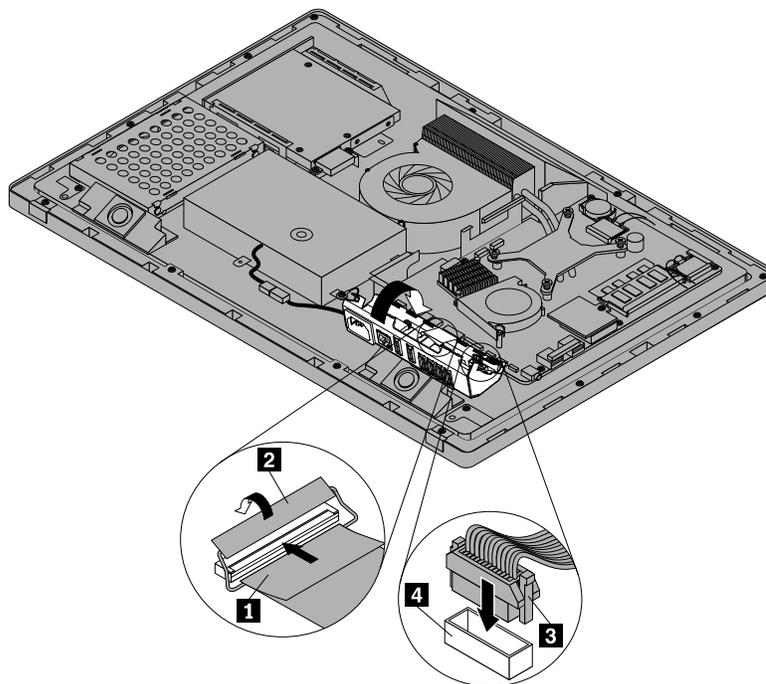
Figure 29. Connecting the HDMI and USB cables
