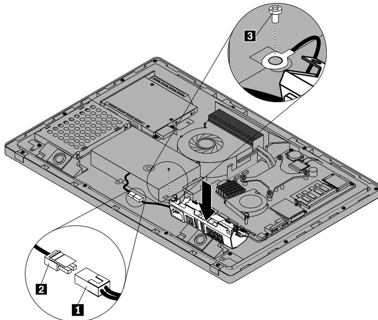
Figure 28. Connecting the power cord cable and securing the earth wire
