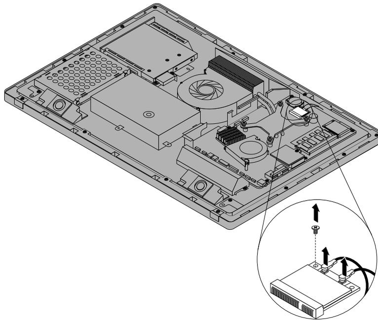
Figure 65. Disconnecting cables and removing the screw from the Wi-Fi card
