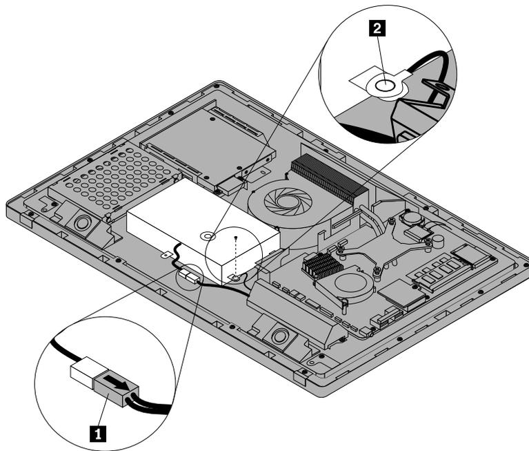
Figure 31. Disconnecting the power cable and earth wire
