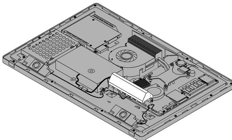
Figure 30. Installing the rear I/O assembly
