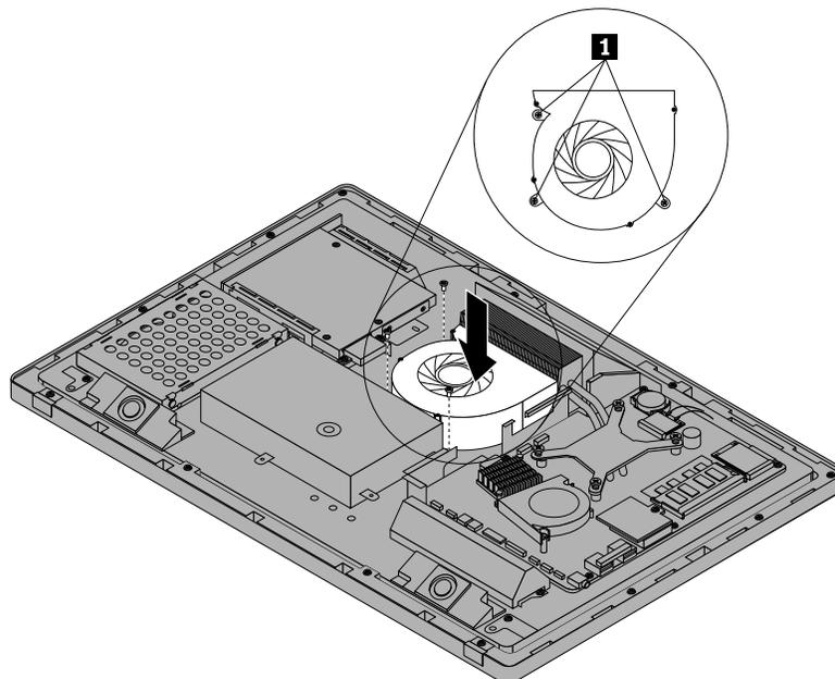
Figure 36. Installing the microprocessor fan
