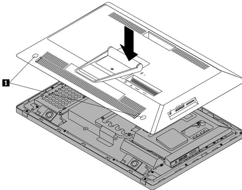
Figure 71. Installing the computer cover
