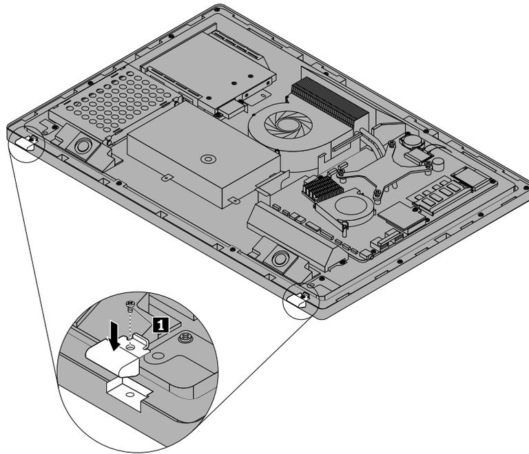
Figure 13. Installing the feet
