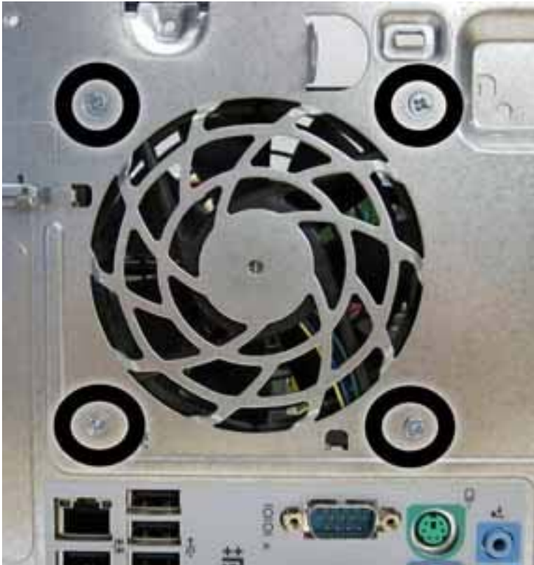
Figure 6-42 Rear fan screws
