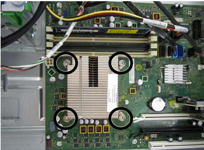
5. Lift the heat sink from atop the processor.
