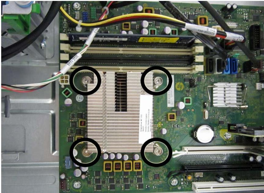
6. Lift the heat sink from atop the processor and set it on its side to keep from contaminating the work area with thermal grease.
