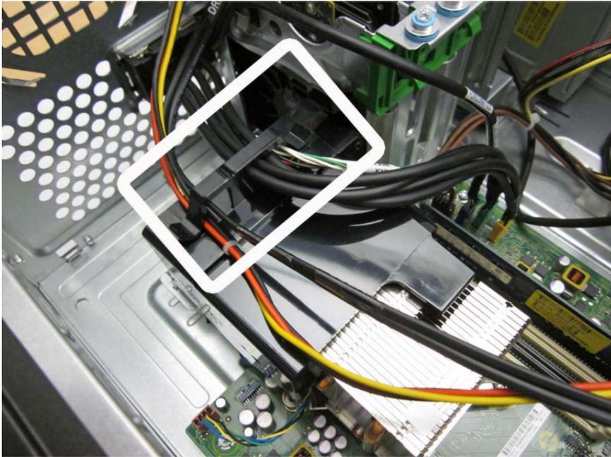
4. Unplug the fan cable from the system board connector labeled CHFAN.
