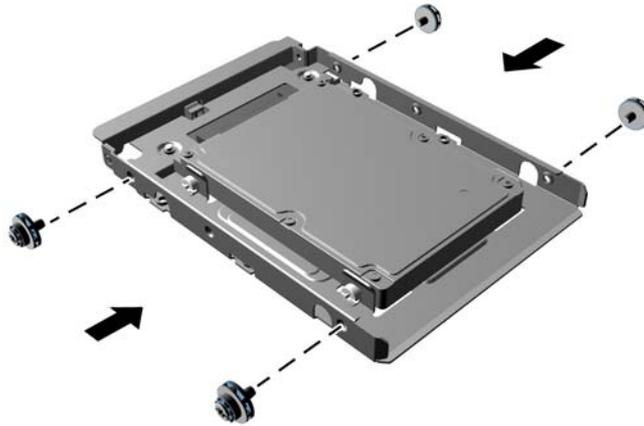
4. Slide the drive into the drive bay, making sure to align the guide screws with the guide slots, until the drive snaps into place. The bottom bay is for the primary hard drive. The upper bay is for an optional secondary hard drive.
