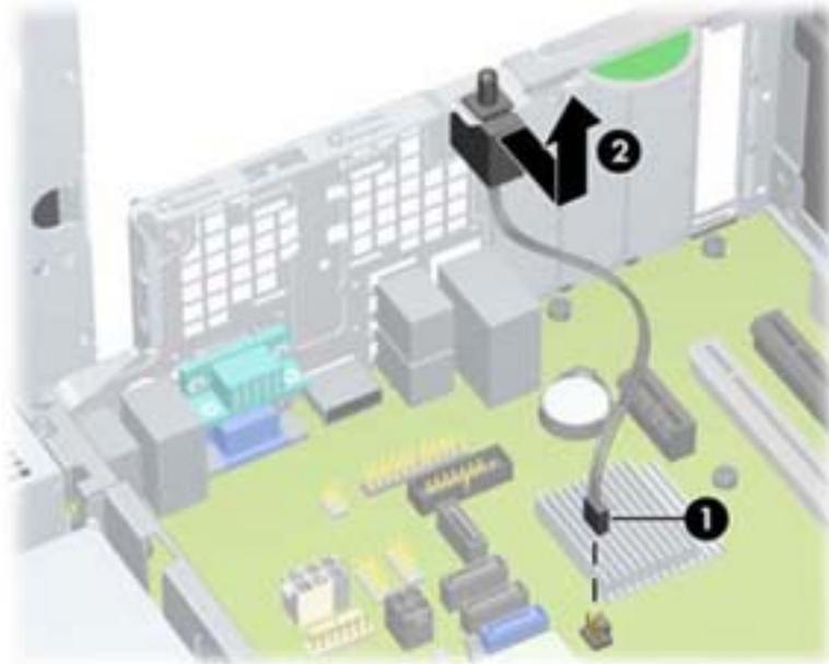
To install the hood sensor, reverse the removal procedure.
