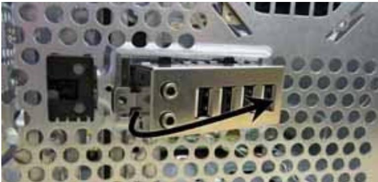
8. Pull the assembly away from the computer while threading the wires through the hole in the front of the chassis.
