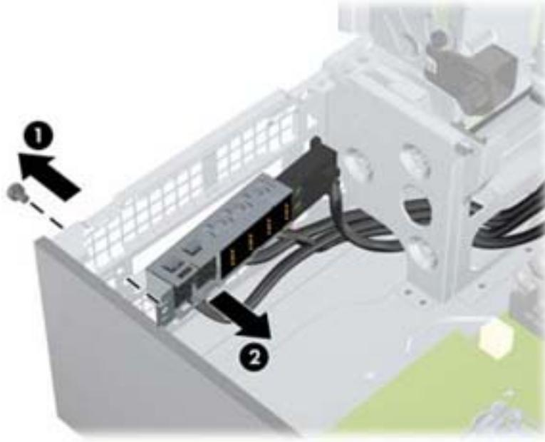
To install the front I/O and power switch assembly, reverse the removal procedure.
