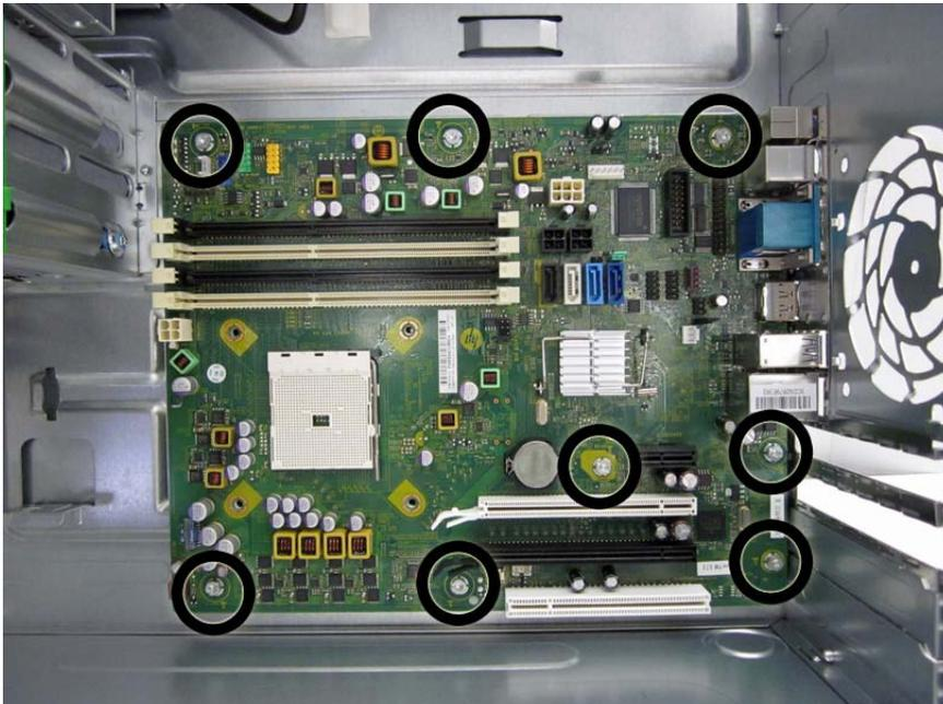
7. Slide the system board toward the front of the computer to disengage the I/O panel, lift the rear of the system board up at an angle, and then lift the system board out of the computer.
