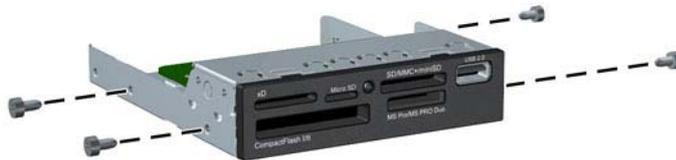
4. Position the guide screws on the drive into the J-slots in the drive bay. Then slide the drive toward the front of the computer until it locks into place.
