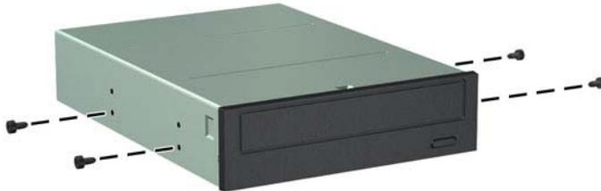
6. Slide the drive into the drive bay, making sure to align the guide screws with the guide slots, until the drive snaps into place.
