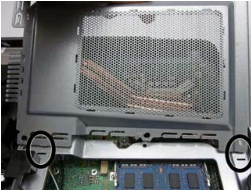
Figure 6-31 installing the heat sink cover
