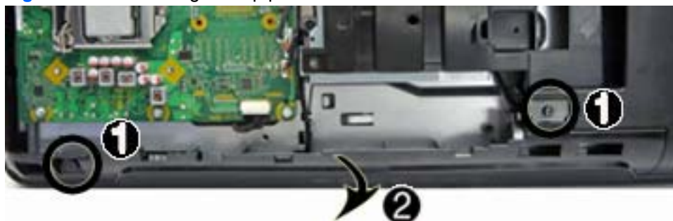
Figure 6-37 Removing the top panel
