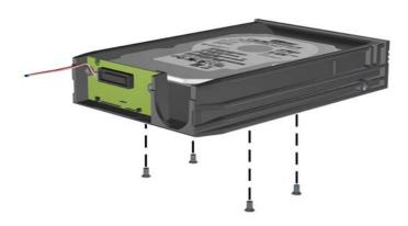
Place the thermal sensor on top of the hard drive in a position that does not cover the label (1) and attach the thermal sensor to the top of the hard drive with the adhesive strip (2).
