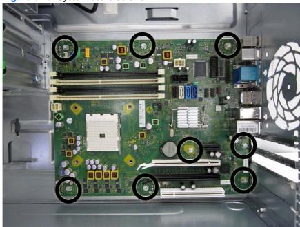
Slide the system board toward the front of the computer to disengage the I/O panel, lift the rear of the system board up at an angle, and then lift the system board out of the computer.
