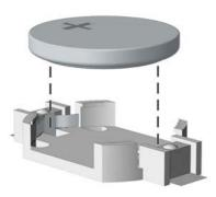
Slide the replacement battery into position, positive side up. The battery holder automatically secures the battery in the proper position.
