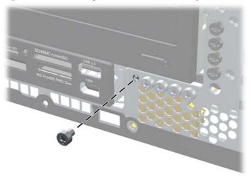
Figure C-7 Retrieving the Front Bezel Security Screw
