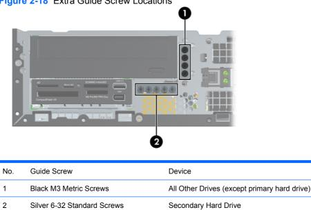
There are at total of five extra silver 6-32 standard screws. Four are used as guide screws for a secondary hard drive. The fifth is used for bezel security (see <u>Front Bezel Security on page 55</u> for more information).
