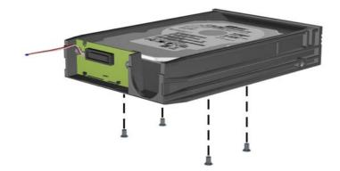
8. Place the thermal sensor on top of the hard drive in a position that does not cover the label (1) and attach the thermal sensor to the top of the hard drive with the adhesive strip (2).
