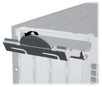
Figure 2-11 Opening the Expansion Slot Retainer
