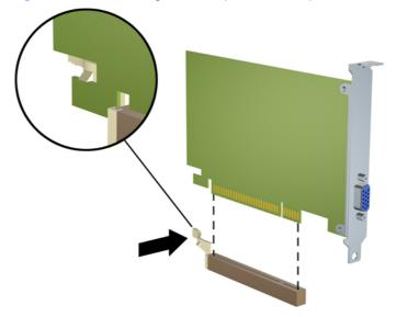
Figure 2-14 Removing a PCI Express x16 Expansion Card
