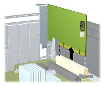
Figure 2-13 Removing a Standard PCI Expansion Card
