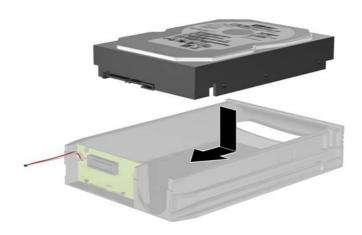
Replace the four screws in the bottom of the carrier to hold the drive securely in place.
