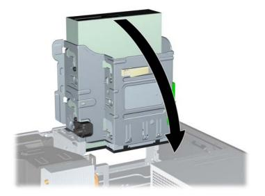
**10.** Press down on the green drive retainer button located on the left side of the drive to disengage the drive from the drive cage (1). While pressing the drive retainer button, slide the drive back until it stops, then lift it up and out of the drive cage (2).
