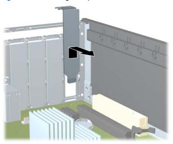
Figure 2-12 Removing an Expansion Slot Cover
