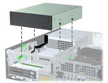
Figure 2-25 Installing the Optical Drive
