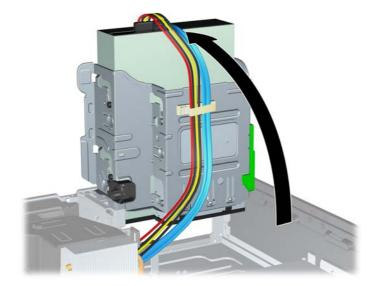
8. If removing an optical drive, disconnect the power cable (1) and data cable (2) from the rear of the optical drive.
