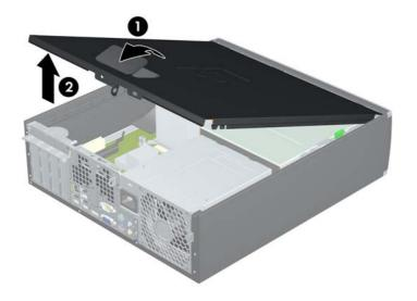
Figure 2-1 Removing the Access Panel
