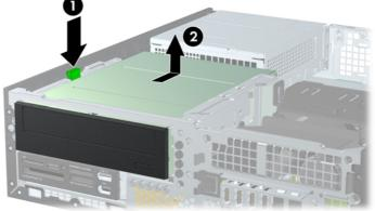
NOTE: To replace the drive, reverse the removal procedure. When replacing a drive, transfer the four guide screws from the old drive to the new one.
