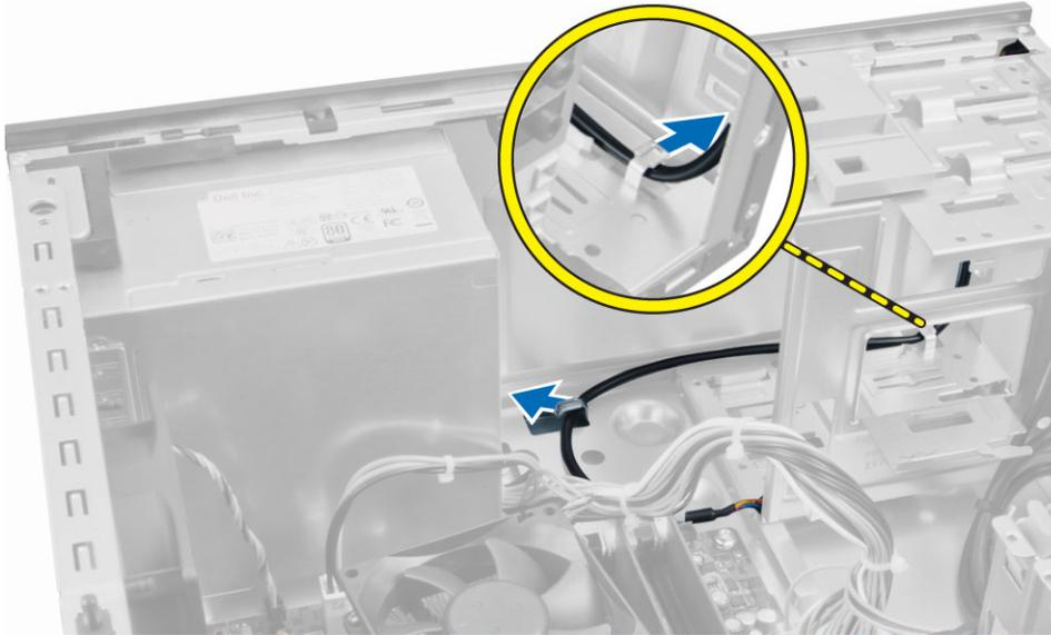
5. Press the clips on both side of the power switch to release it from the chassis and, slide to remove the power switch along its cable from the computer.
