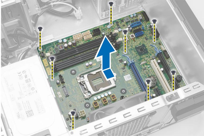
5. Tilt the system board at 45–degrees, and then lift the system board out of the computer.
