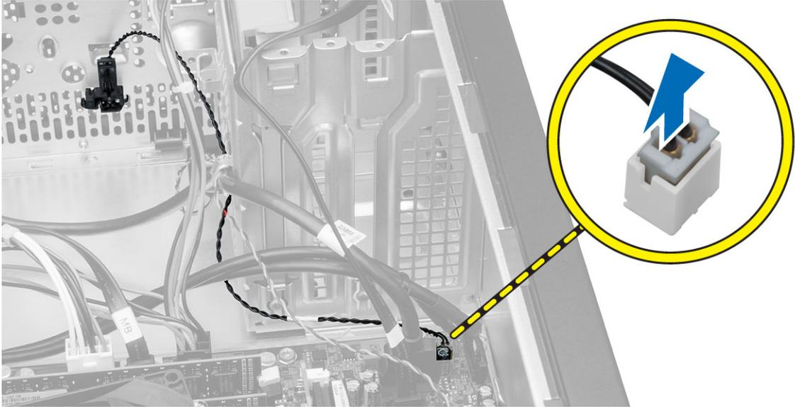
4. Release the thermal-sensor cable from the chassis clip.
