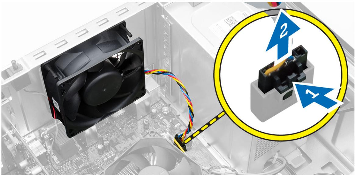
4. Pry and remove the system fan away from the four grommets securing it to the back of the computer.
