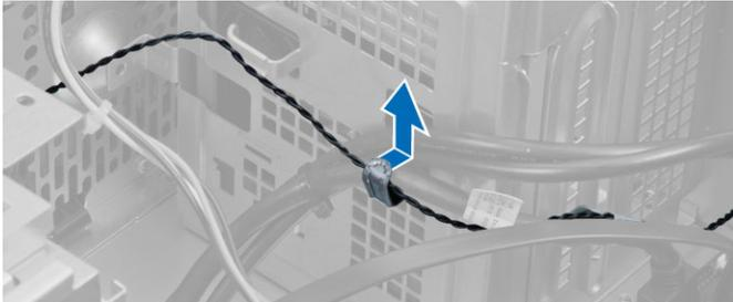
5. Press the tabs on both sides to release and remove the thermal sensor away from the chassis.
