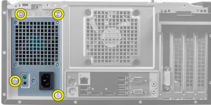
5. Push in on the blue release tab beside the power supply, and slide the power supply towards the front of the computer. Lift and remove the power supply out of the computer.
