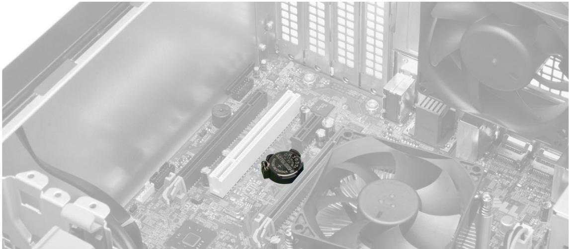
4. Press the release latch away from the battery to allow the battery to pop-up from the socket and lift the coin-cell battery out of the computer.
