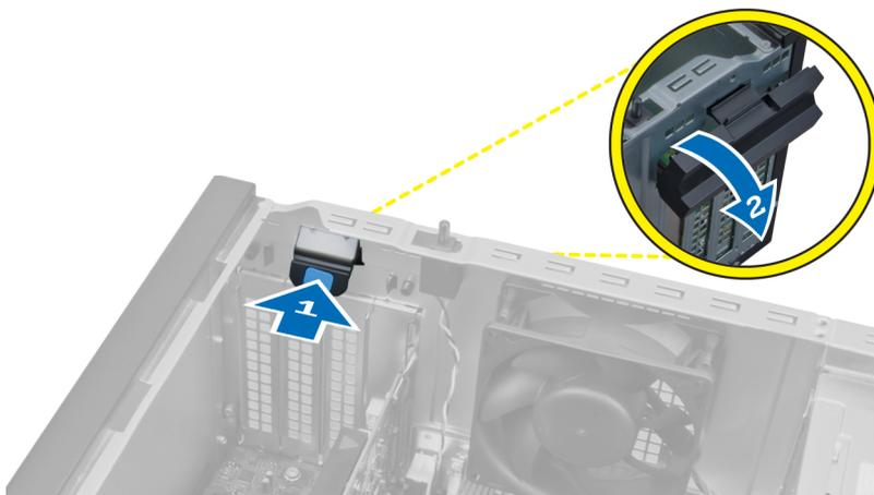
4. Pull the release lever away from the PCI x16 card until you release the securing tab from the dent in the card. Lift the card out of its connector and remove it from the system board.
