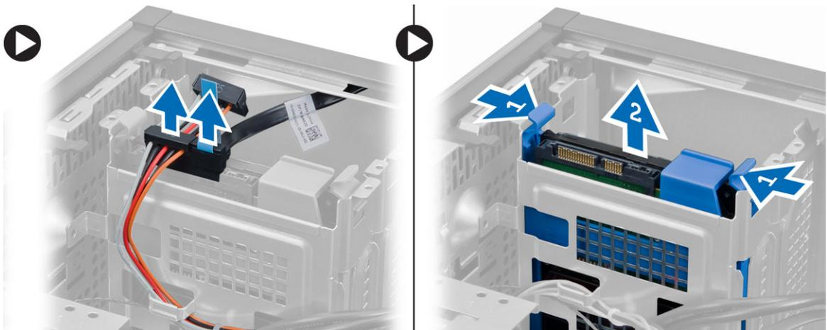
4. Flex the hard-drive bracket and remove the hard drive from the hard-drive bracket.
