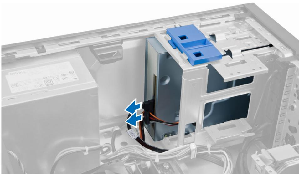
4. Slide and hold the optical-drive latch to unlock the optical drive and pull the optical drive out of the computer.
