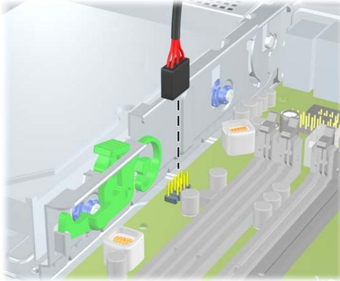
**Figure 2-31** Disconnecting the Media Card Reader 1394 Cable
