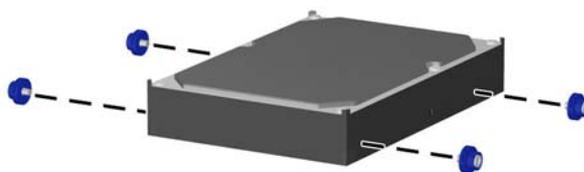
12. Align the guide screws with the slots on the chassis drive cage, press the hard drive down into the bay, then slide it back until it stops and locks in place.
