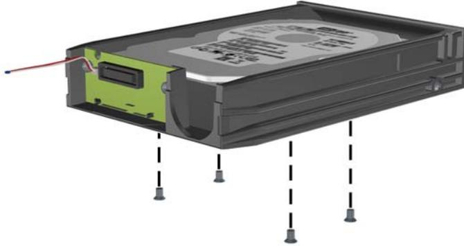
5. Slide the hard drive back to disconnect it from the carrier then lift it up and out of the carrier.
