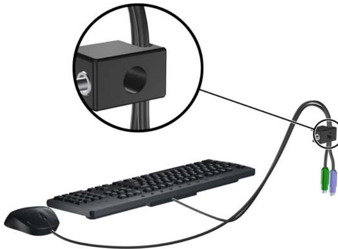
3. Remove the left screw that secures the computer access panel to the chassis and screw the lock to the chassis using the screw provided.
