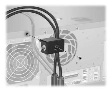
3. Insert the plug into the lock **①** and push the button in **②** to engage the lock. Use the key provided to disengage the lock.
