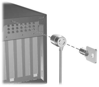
Installing a Cable Lock
