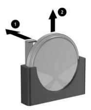
Removing a Coin Cell Battery (Type 3)
