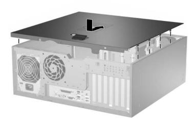
Replacing the Computer Access Panel
