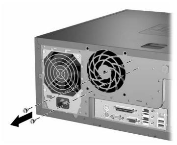
Removing the Smart Cover Lock Screws
