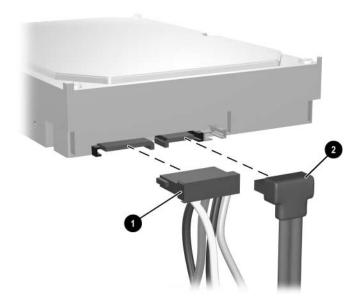
Connecting the Power Cable and Data Cable to a SATA Hard Drive
