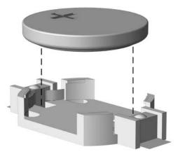
Removing a Coin Cell Battery (Type 1)
