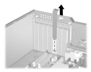
Removing an Expansion Slot Cover
