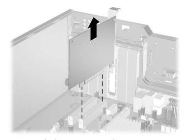
Removing a Standard PCI Expansion Card
