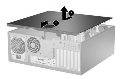
Removing the Computer Access Panel
