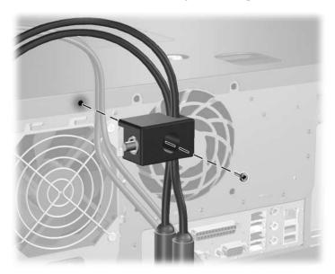
4. Insert the plug end of the security cable into the lock **①** and push the button in **②** to engage the lock. Use the key provided to disengage the lock.
