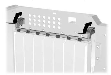
Opening the Expansion Slot Retainer
