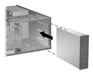
Installing a Drive in the Minitower Configuration
