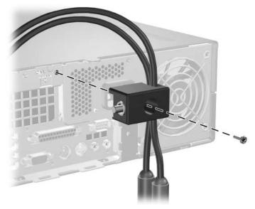
3. Screw the lock to the chassis using the screw provided.
