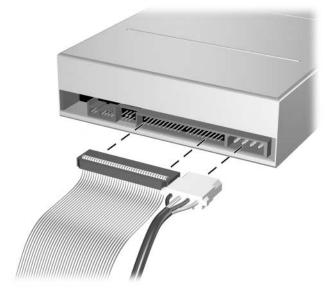
Disconnecting the Power and Data Cables
