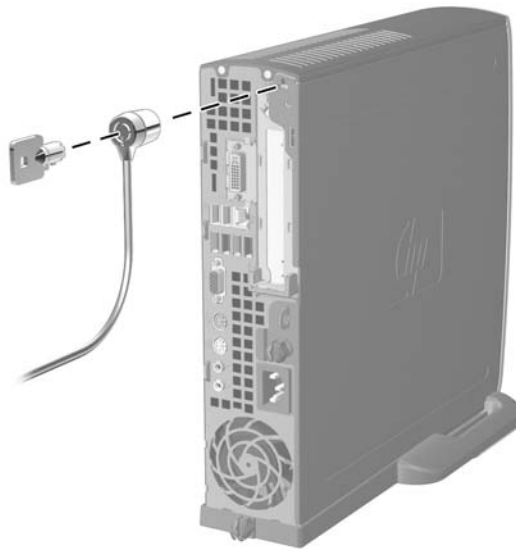
Installing a Cable Lock
