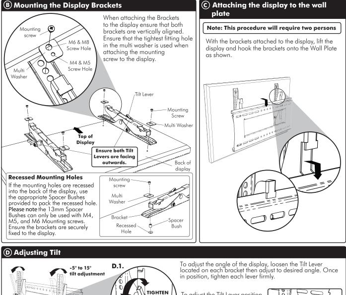
To adjust the Tilt Lever position without tightening or loosening the lever, pull the lever as shown to dis-engage the ratchet mechanism and rotate the lever into the desired position.
