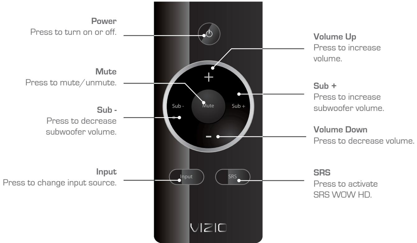
For best results, point the remote at the right side of the Sound Bar. The sensor is located there.
