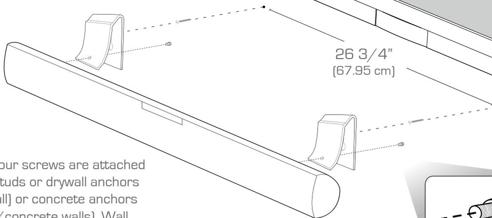
2 Be sure your screws are attached to wood studs or drywall anchors (for drywall) or concrete anchors (for brick/concrete walls). Wall mounting hardware is not included.
