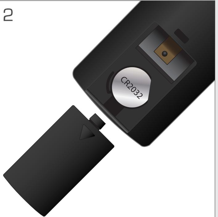
Replace the old battery with a new CR2032. Be sure that the + sign on the battery is facing up.
