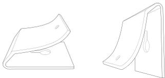
Remove the screw from the Sound Bar stands and rotate as shown.
