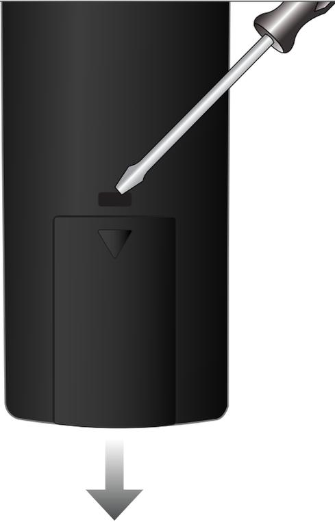
Insert a flat-head screwdriver into the slot as shown. Gently push down on the tab, then press and pull downward on the battery cover to open.
