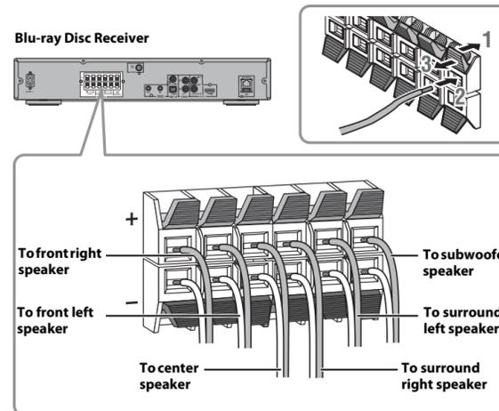
Connect the center, surround, subwoofer speaker cables to the Blu-ray Disc Receiver. Make sure you connect the speakers with the correct polarity: positive (+) cables to positive (+) terminals, and negative (-) cables to negative (-) terminals.
