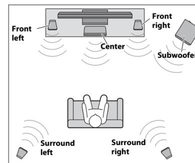
The front and surround speakers are identical, so it does not matter which one you use in each position. Position the speakers as shown. See the owner's manuals for more information on installing the speakers. When placing the speakers on a flat surface, affix the included non-skid pads to the corners of the speaker undersides.
