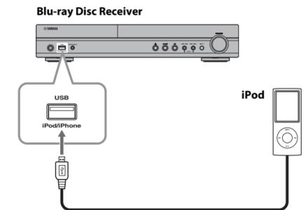
Use an additional USB cable to connect the iPod/iPhone to the Blu-ray Disc Receiver, as shown.
