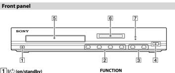
1 I/ (on/standby) Turns on the unit, or sets it to standby
