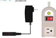
\*When selecting a surge protector, it is STRONGLY recommended to use one that is UL-1449 rated, for a clamping voltage of 330 or lower, a Joule rating of at least 400 and a response time of 10 nanoseconds or less.
