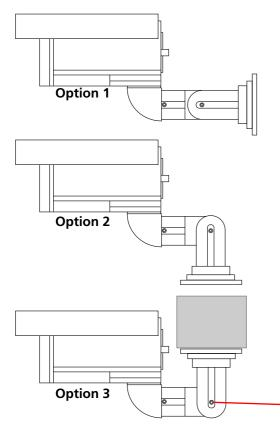
There are three ways that you can mount the PRO-780: to a wall (1, recommended) or to a horizontal surface, either above (2) or suspended (3, requires additional hardware).
