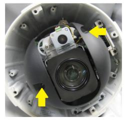
2. The micro SD/SDHC card is inserted in direction of the following picture.( The contacts face downward.)
