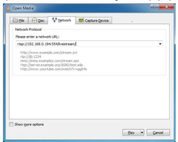
3. The address format is rtsp://<ip address>:<rtsp port>/<RTSP streaming access name>. For example, rtsp://192.168.0.194:554/livestream
