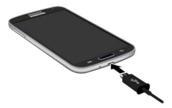
3. When charging is finished, remove the USB cable from the charger/accessory jack on the phone.
