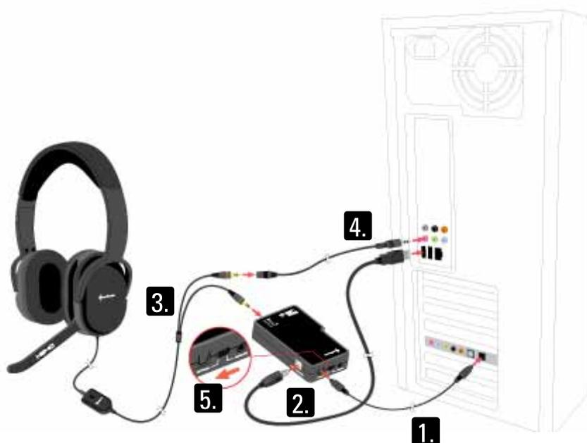
1. Connect the optical cable to the PC and the SCU.
