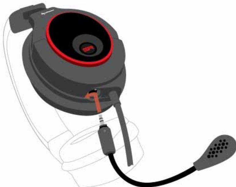
The microphone will only fit in one direction. Both the microphone and the headset bear markings. Turn the microphone until its marking and the marking on the headset are opposite to each other. Press the microphone into the connector of the headset and turn it to the front and into the desired position.
