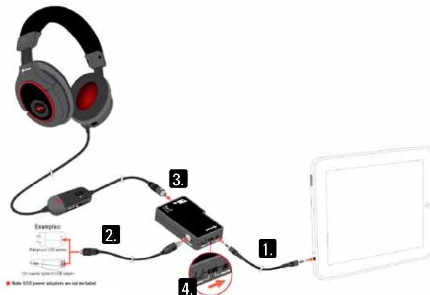
1. Connect the stereo connection cable to the device and the SCU.
