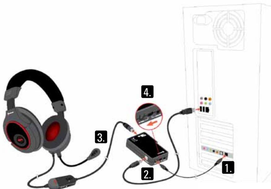
1. Connect the optical cable to the optical connector of your PC sound card and the SCU.
