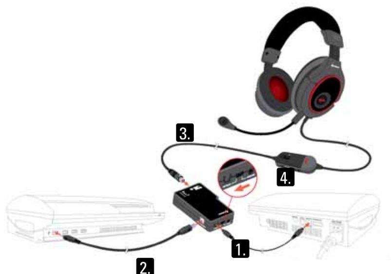
1. Connect the optical cable to your console and the SCU.
